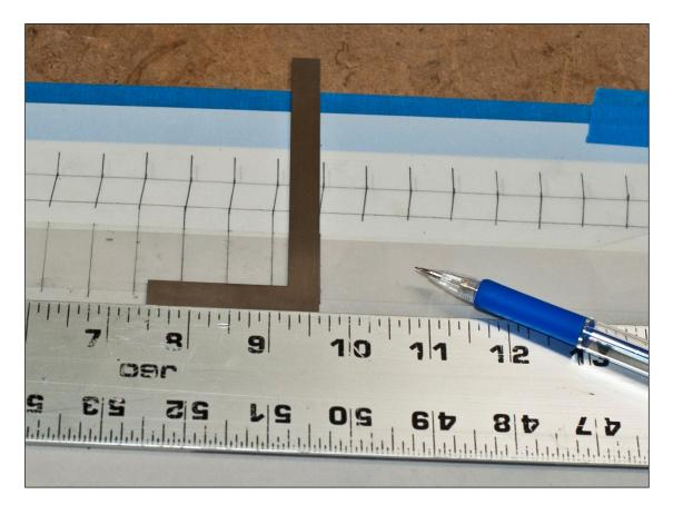
Lay a 25mm or 1" wide strip of mylar on top of the mylar you have been working on. Tape down so that the strip is parallel to the note line. WNG supplies a scale stick kit with a mylar pencil, square and 25mm wide strips of mylar for your convenience.
