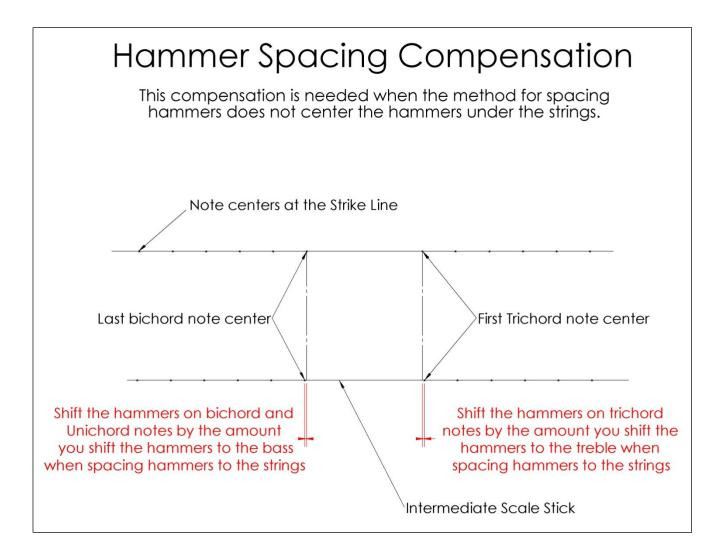
On the overwhelming majority of pianos, the Soft Pedal shifts the action towards the treble so that trichord hammers will miss one string. Because of this there are at least two ways to space hammers to the strings.
