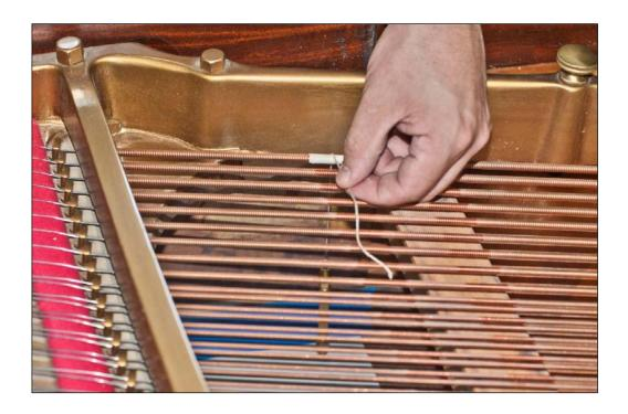
Use the piano technician's plumb bob to transfer the mark on #1 bass string down to the mylar in the keybed.
