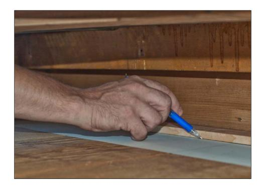
Use a straight edge and a mylar pencil to draw a line between the note #1 and note #88 strike points on the mylar.
