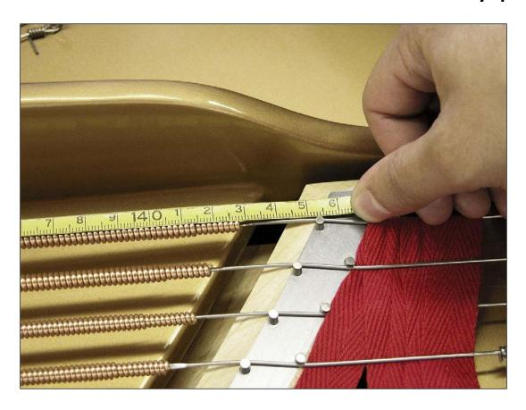
Start by measuring the speaking length for note #1. Use a millimeter tape measure for this task. Since you want to calculate using these numbers, use a measuring device that is decimal to begin with. While you can use fractional English measurements and then convert them to decimal, unneeded work is involved and not very sensible.
