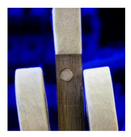
When glued on square, because of hammer front to back movement, clearance will always be a problem. Above you can see what happens when angled hammers are glued on square.
