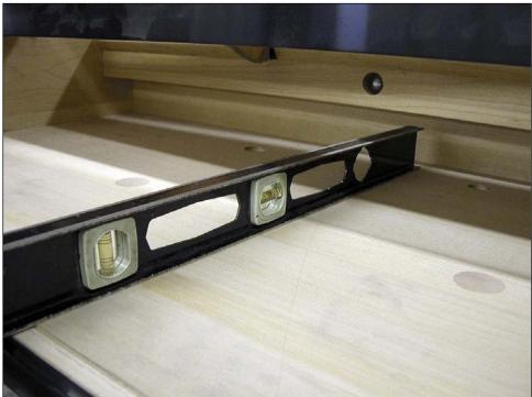
Use a level on the keybed to make sure that the piano is sitting level. It is necessary to level the keybed bass to treble and front to back.
