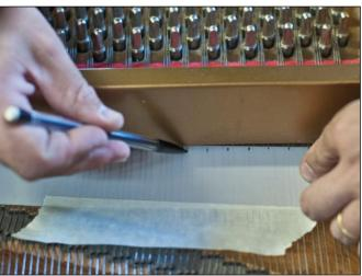
In the high treble there is not enough room to use a piece of mylar with a line drawn on it as in the lower sections of the piano. Instead cut an edge on a piece of mylar that is straight. That will serve as your line. Cut the ends as before and tape the mylar onto the strings so the edge is on the strike line marks on the end of section notes.
