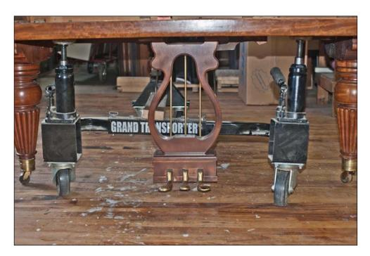
Another way to level a piano is using the hydraulic jacks in a Grand Transporter.
