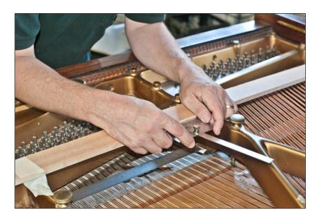
To measure the string angles, you need a straight edge aligned to the strike line to measure from. Place a straight edge on top of the plate bars. Using two small squares align the straight edge to the strike line marks you placed on tape on the strings earlier. Tape the straight edge into place with masking tape so it cannot move while you are measuring the string angles.
