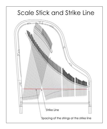
A strike line is a theoretical line that runs across the piano. The intersection between this line and the strings defines the point where the hammer hits the string. Sometimes, due to poor execution during the making of the plate, the strike line in actual practice is less then straight. You can be assured, however, that the piano was designed with a straight strike line.
