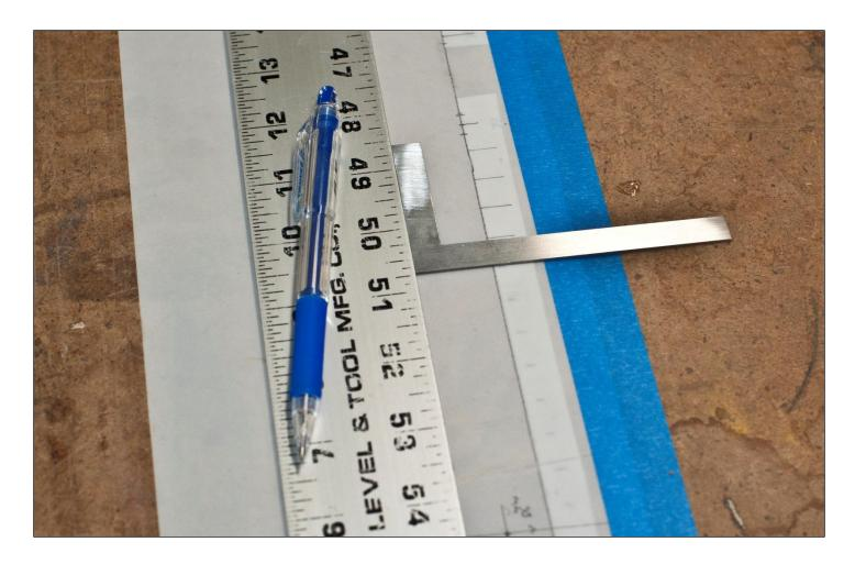
With the section mylar under the keybed mylar, you will be able to see the locations of each note. Mark these locations on the keybed mylar.
