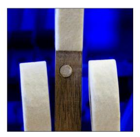
Traditionally, piano makers have tilted the hammer gluing so as to create clearance. The pictures show clearly how effective the technique is in creating clearance for the hammers.
