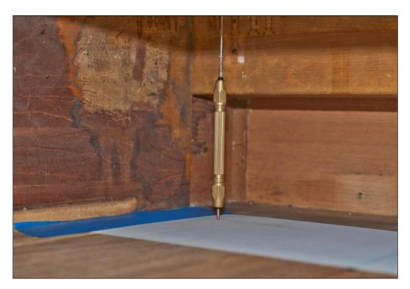
Make a mark on the mylar where the plumb bob points to mark the strike location for note #1.
