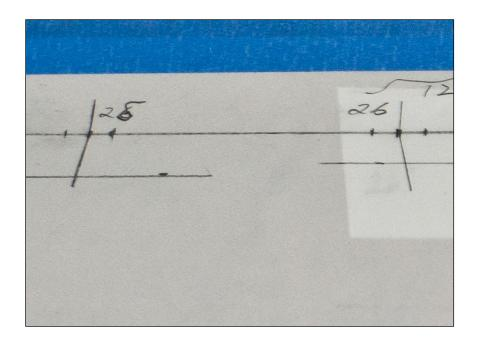
Here we have drawn the hammer front to back motion line for the bass and the treble.
