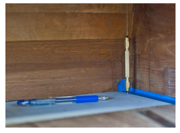
This is the piano technician's plumb bob. It is just a pin vise that every piano technician has in his or her tool kit. Put a center pin in one end, use a small size. In the other end clamp to a fairly thin fishing line.
