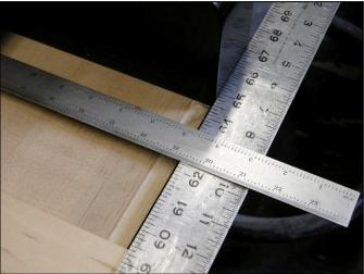
Measure from the arms of the piano to the strike location at note 88. Mark this on the mylar at note 1.
