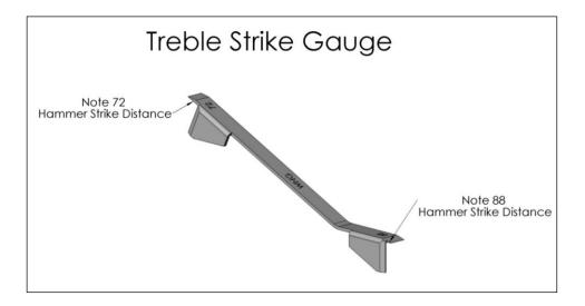
The Treble Strike gauge is a WNG tool that facilitates finding the proper strike point for notes 72 and 88.
